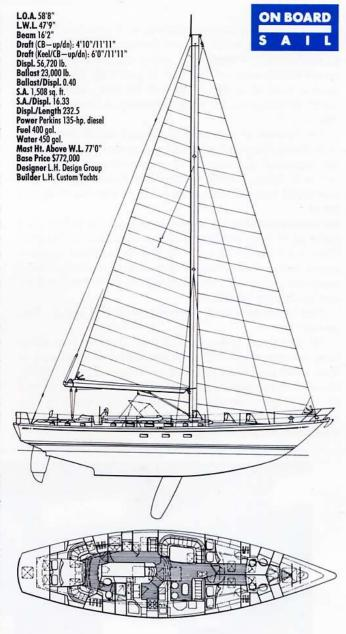
forestay, and a fully powered electric self-tailing Barient winch package. In keeping with the goal of full control of the yacht from the helm, essential lines lead to the cockpit, and winch-control buttons are within reasonable reach of the helm. While Little Harbor has not taken the leap toward fully automated, joystick control, this is about as close as you can get to comfortable, shorthanded sailing without a computer.
