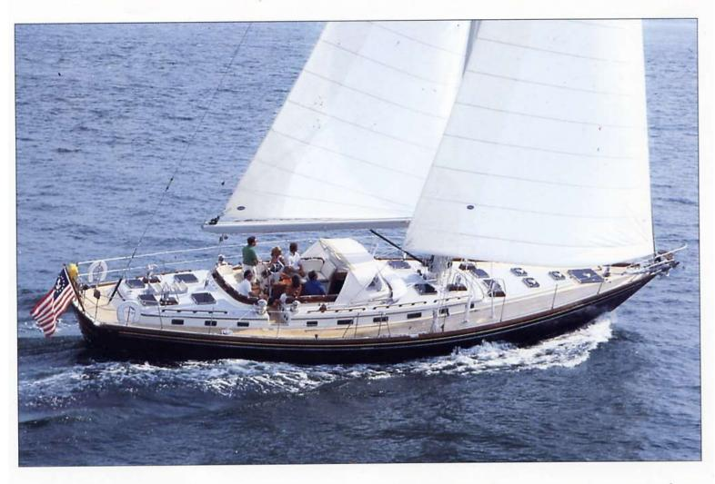
0.40, it is effectively higher when you consider the centerboard trunk structure, heavy hull scantlings, machinery and batteries mounted low in the hull. So in a seaway she will have an easier motion (contrasted with the sharp motion of light, deep-keeled boats) and carry her sailplan well.
